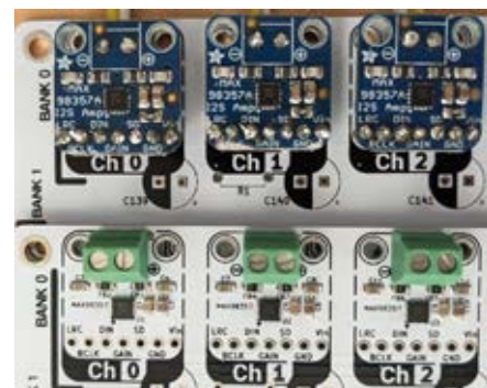
Figure 2. Two Frugal Boards side by side with the two different integration: direct MAX98357A audio codec integration (bottom) or using Adafruit breakout boards (top).
