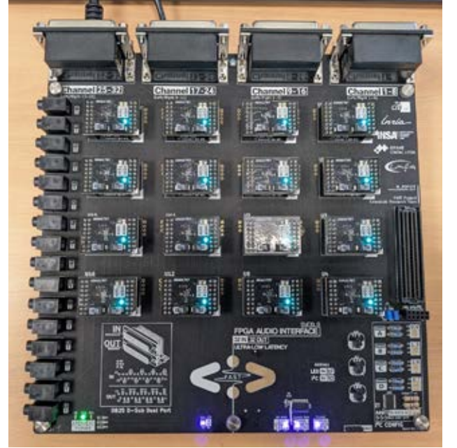
Figure 4. 32 Channels Ultra Low Latency FPGA interface stacked on the Genesys ZU-3EG. The motherboard embeds 16 breakout boards with ADAU1787 codecs.
