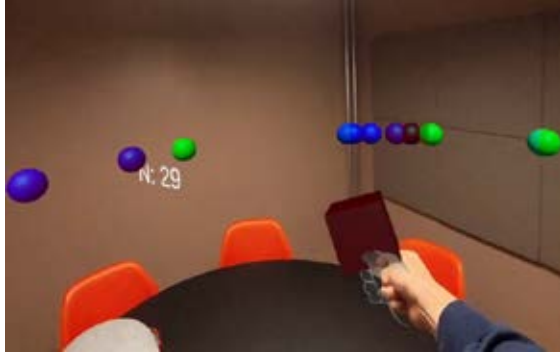
Figure 2: Screenshot for the mixed reality application taken in the Meta Quest 3 . The audio sources are represented by coloured spheres orbiting around an interactive cube that can be moved using any user’s hand. In this scene, 29 objects were instantiated, but some are not visible due to the field of view limit.
