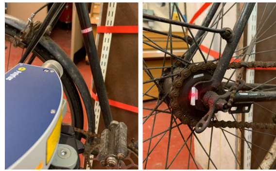
Figure 10. A practical example of the LDV in use for sound design applications: capturing the subtle mechanical sounds of a vibrating bike frame.
