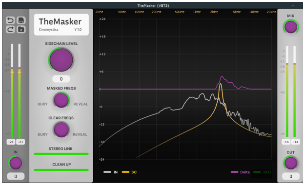
Figure 2. TheMasker Graphical User Interface. In this example, a sine wave masking some noise is visible, with the correction curve boosting all noise components below a spreading window.
