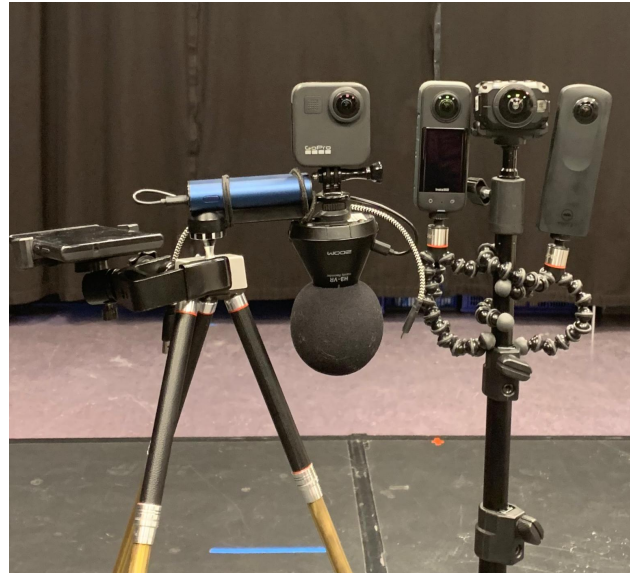
Figure 2. The experimental setup: four 360-degree cameras (left to right: GoPro MAX, Insta360 X3, Garmin VIRB 360 and Ricoh Theta S). A Samsung Galaxy S23 Ultra mobile phone captured sound and light levels.
