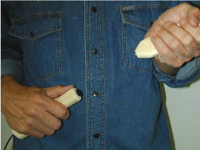
Figure A.4: Control sticks for playing the VAG. Right-hand stick (on the left) includes an acceleration sensor as well as a small loudspeaker to send the distance measurement pulse. Left-hand stick (on the right) receives the pulse by an electret microphone.
