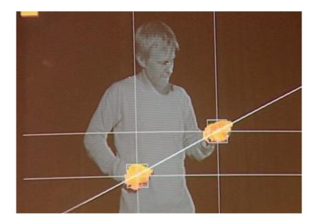
Figure A.5: Camera tracking of hand positions (orange gloves), as seen by the computer.
