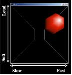
Figure 7.2: Two different examples of the Expressiball giving visual feedback of musical performance. Dimensions used in the interface are: X = tempo, Y = sound pressure level, Z = spectrum (attack time and spectrum energy), Shape = articulation, Colour = emotion. The left figure shows the feedback for a sad performance. The right figure shows the feedback for an angry performance.
