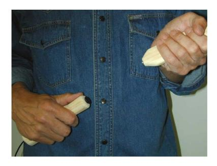
Figure A.4: Control sticks for playing the VAG. Right-hand stick (on the left) includes an acceleration sensor as well as a small loudspeaker to send the distance measurement pulse. Left-hand stick (on the right) receives the pulse by an electret microphone.
