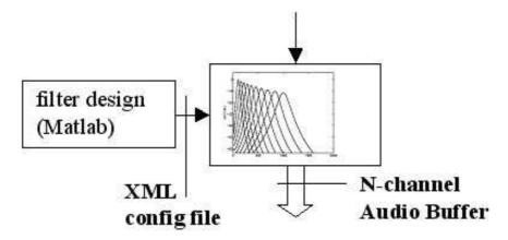
Figure 6.4: Design of the auditory filter bank through the Matlab Auditory Toolbox
