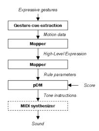
Figure 7.4: Overall schematic view of a home conducting system.
