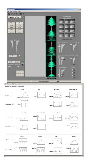
Figure A.1: Skipproof graphical user interface (left) and synthesised techniques (right). The GUI contains a combination of standard controllers found on turntables and mixers, and novel controllers such as technique triggers, visual representation of sound, sliders for changing control parameters, and more. The synthesised techniques are saved as sets of two tables; the upper is the record movement and the lower is the crossfader movement.
