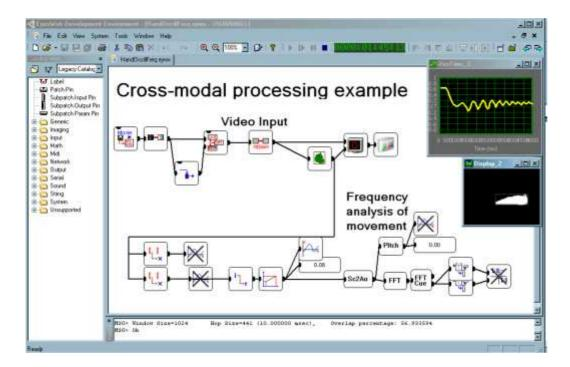
Figure 6.7: An example of EyesWeb application for cross-modal analysis of movement: the hand vertical displacement, measured from the video signal, is converted into the audio domain and analyzed through a pitch detector.
