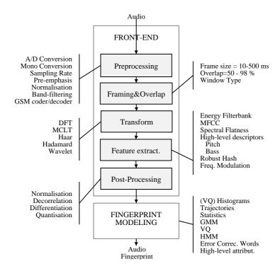
Figure 3.1: Fingerprint Extraction Framework: Front-end (top) and Fingerprint modelling (bottom).
