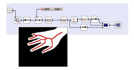
Figure 6.8: An EyesWeb 4 patch extracting the skeleton of a hand touching a TAI
