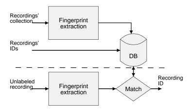
Figure 3.7: Content-based audio identification framework
