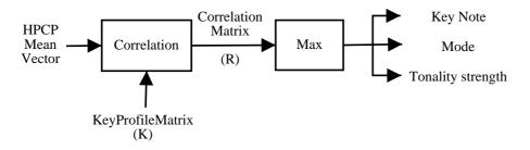
Figure 3.5: Block Diagram for Key Computation using HPCP
