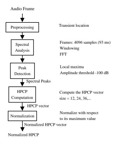
Figure 3.4: Block Diagram for HPCP Computation
